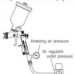
Pulling the trigger of the gun with the pattern adj. Set and fully opened adjust the air regulator in the spray booth to obtain 1.0~1.3 bar (14~18 PSI) at the gun inlet as issued on specifications table ahead. In this way the gun will atomize within 0.7 bar (10 PSI) inside air cap.
