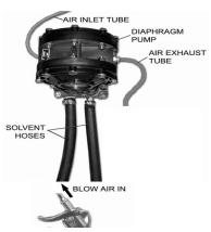
This procedure will also clear a blockage in the fluid line for the wash gun.
